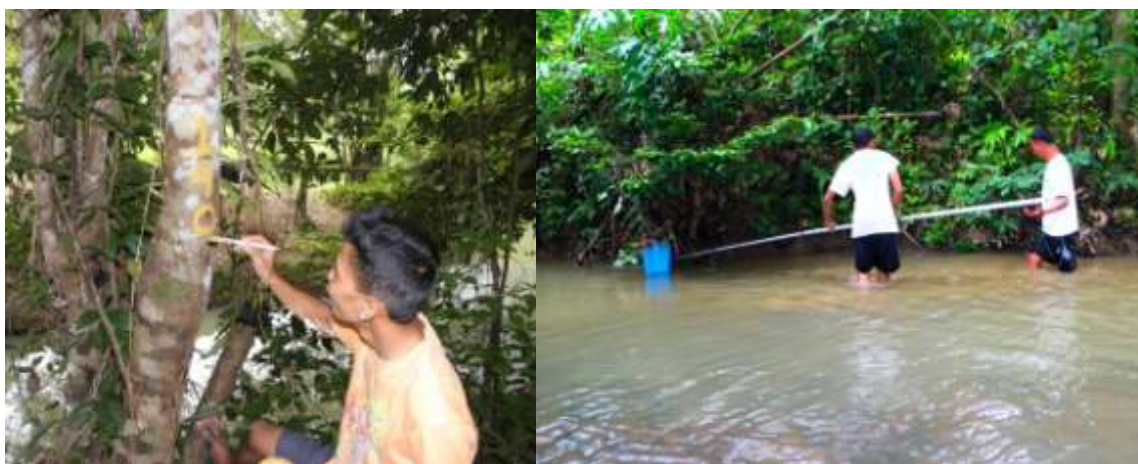
Plate 13: The streams are marked at 10-meter-intervals and physical and chemical measurements are taken (left). Team members measuring stream width, depth and water current speed (right).
